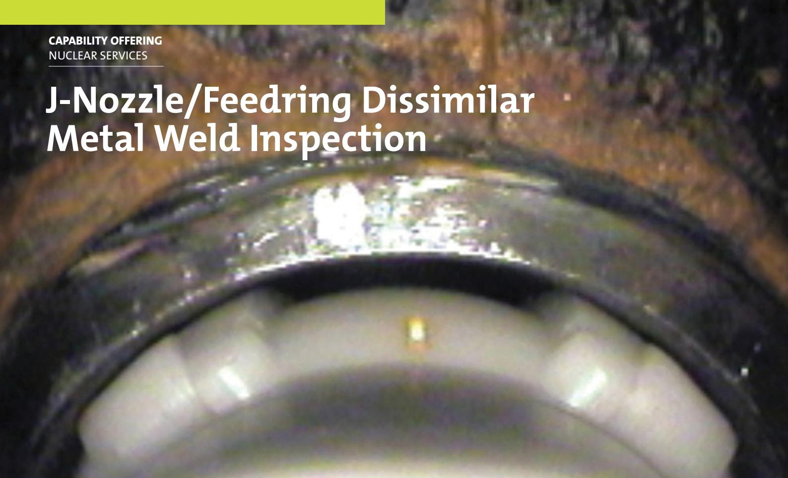
The Brooks J-Nozzle inspection tool is an exclusive visual inspection solution, ensuring customers have access to more inspection data, faster and safer than ever before. Inspect a full 360° of the J-Nozzle weld, while recording location feedback for trending and more efficient maintenance planning.
