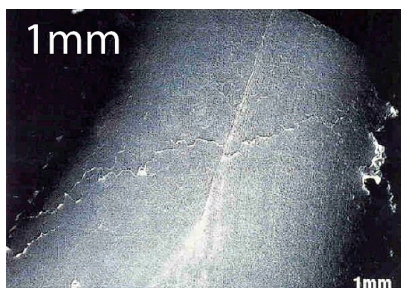
1- Intergranular cracking in replicated surface
