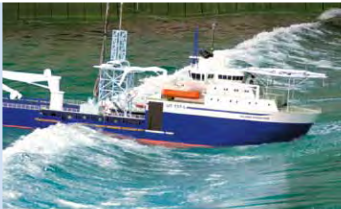
The Rolls-Royce designs, types UT and NVC, are tested in model tanks to maximise speed and sea-keeping according to the clients’ requirements.
